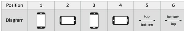
Fig. 6. Rotating a sensor module (smartphone) to six different positions on a flat surface.
