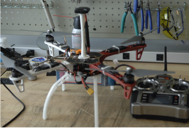
Fig. 3. Custom-built rotary wing UAV.
